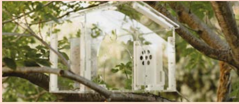
▲ Smart Bird Feeder. Follow the instructions at Coral's website to build a smart birdhouse that records birds and deters squirrels ( magpi.cc/smartbird )
